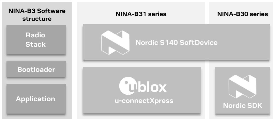
Figure 2: NINA-B3 software structure and available software options
