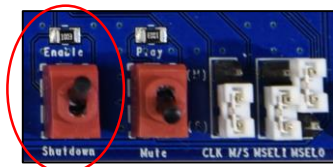
Figure 8. Left toggle switch set to “enable” position.
