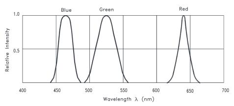
Fig.1 RELATIVE INTENSITY VS. WAVELENGTH
