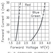
Fig.2 FORWARD CURRENT VS. FORWARD VOLTAGE
