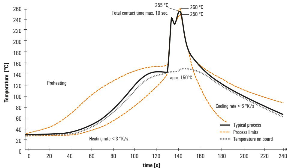
**Wave soldering profiles**
