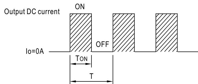
$$\text{Duty cycle}(\%) = \frac{T_{ON}}{T} \times 100\%$$
