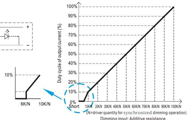
Note : 1. Min. duty cycle of output current is about 0.15%, and the dimming input is about  $6K\Omega$  or 0.6VDC, or 10V PWM signal with 6% duty cycle.
