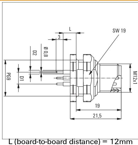
**Front panel section**  $D1 = 5,0 \text{ mm}$
