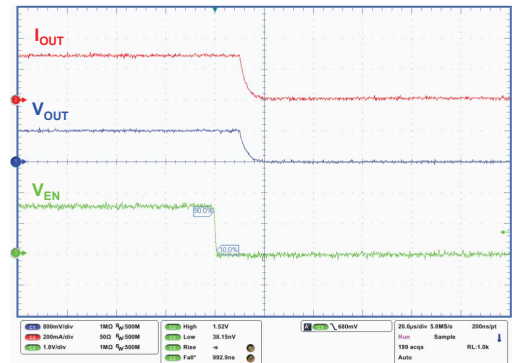
Figure 36. Turn-off by enable
