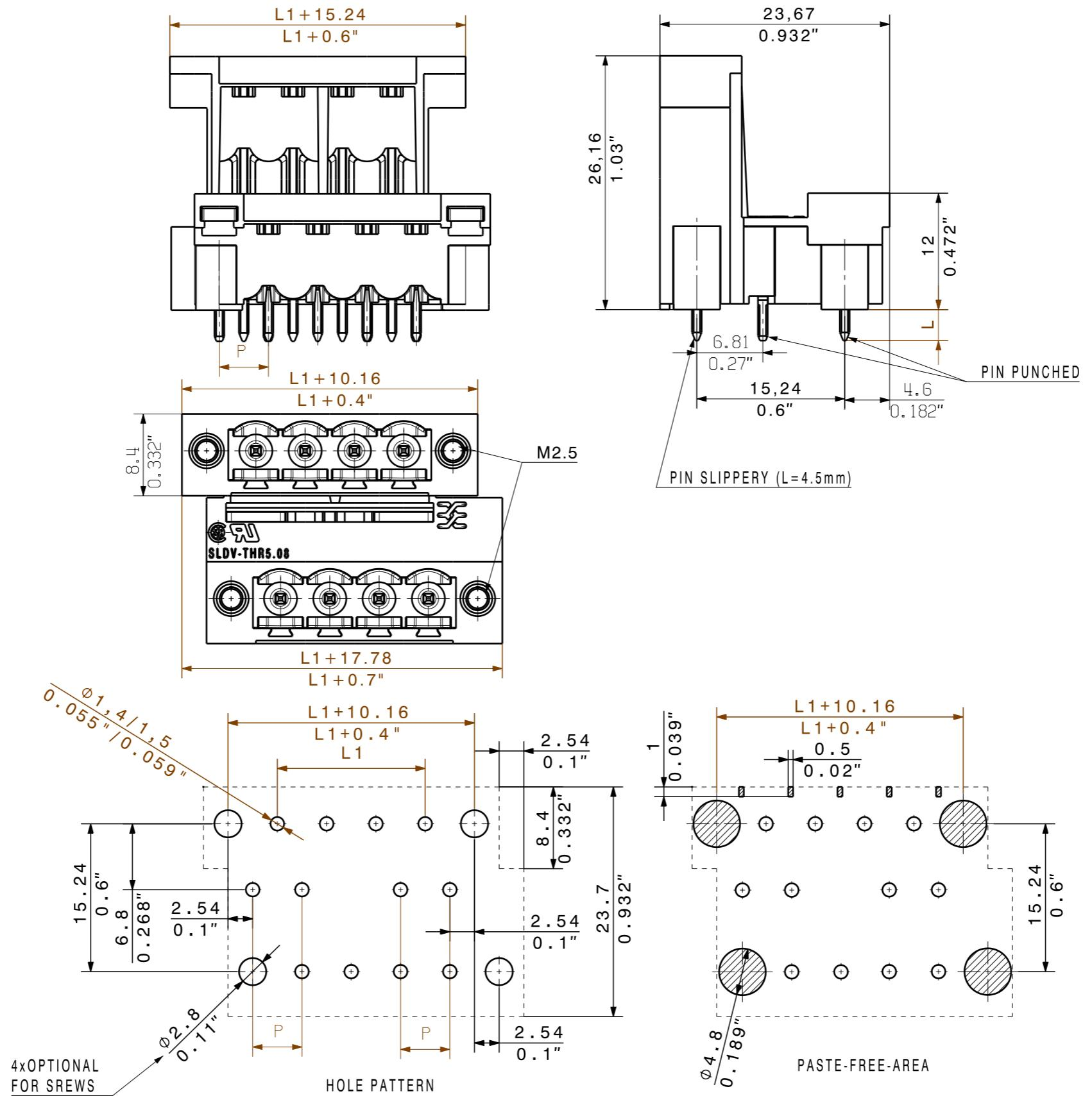
For the mounting of PCBs, it should be noted that the rated data given in the catalogue relates only to the connection elements. The necessary creepage and clearance paths must be observed in connection with the respective applicant in accordance to VDE 0110. The current-carrying capacity and pitch tolerance is to be determined according to DIN IEC 326 part 3 very fine.
