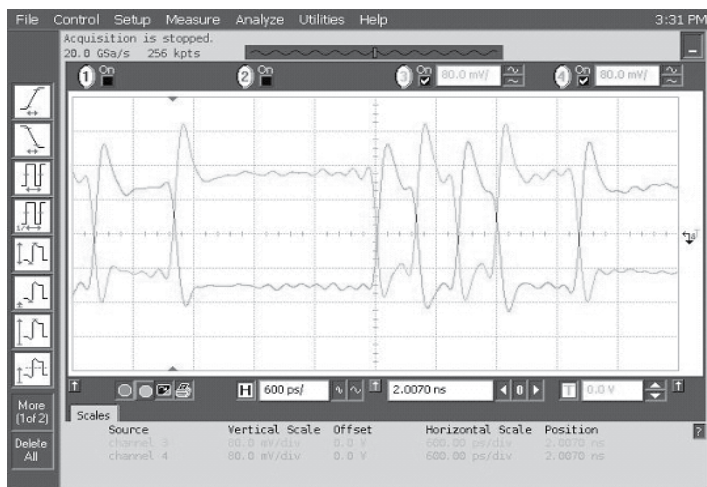
Data Waveforms, 2.5Gbps (left) & 5.0Gbps (right)
