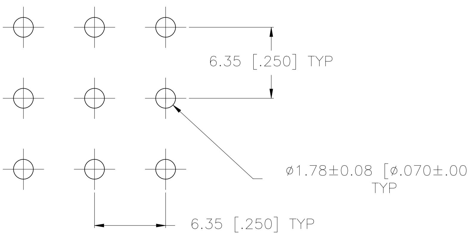
RECOMMENDED LAYOUT FOR 1.58 [.062] THICK PC BOARD
