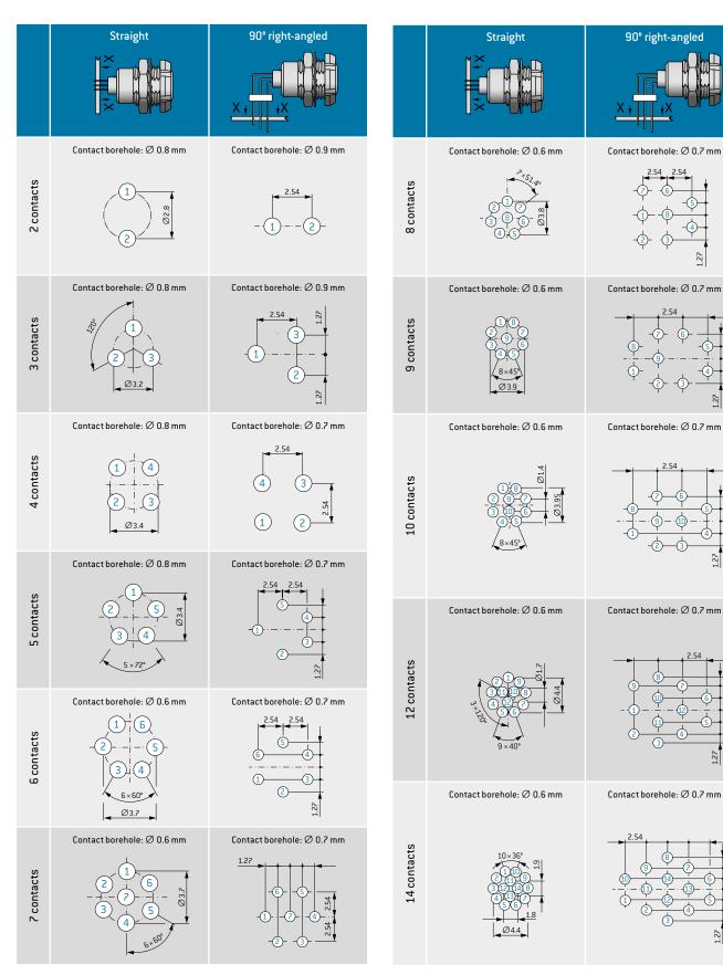
All specifications are only valid for socket inserts, pin inserts on request. Further PCB layouts upon request
