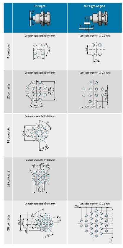
All specifications are only valid for socket inserts, pin inserts on request. Further PCB layouts upon request
