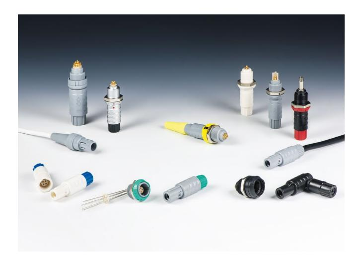
The ODU MEDI-SNAP® combines distinctive coding options with 2,000 / 5,000 mating cycles depending on the connector style. The efficient plastic connector is available both with user-friendly Push-Pull locking and the easy-to-release Break-Away function, which comes as a premolded plug & play solution. The ODU MEDI-SNAP® portfolio offers also a High-Voltage solution for up to 1,000 V AC / 16 A including a hot-plugging prevention.
