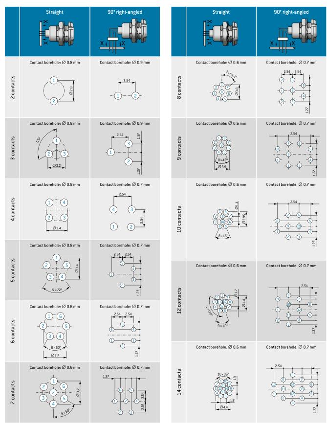
All specifications are only valid for socket inserts, pin inserts on request. Further PCB layouts upon request
