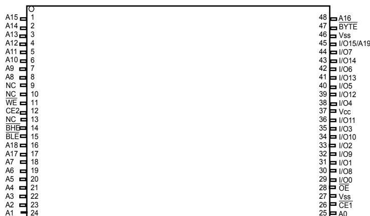
Figure 3. 48-pin TSOP I pinout (Top View) [1, 3]
