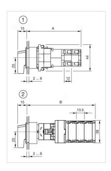
1 = Kraus & Naimer switching element A = (Number of stages x 12) + 66.5 mm 2 = Santon switching element B = (Number of stages x 13.5) + 65.5 mm
