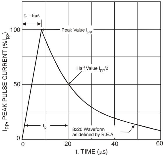
Figure 3 Pulse Waveform
