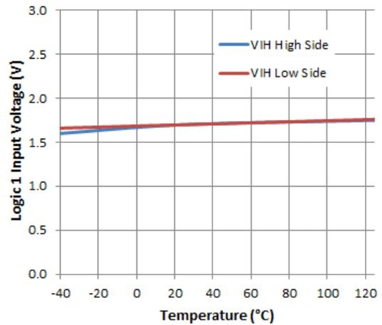
**Figure 21.** Logic 1 Input Voltage vs. Temperature
