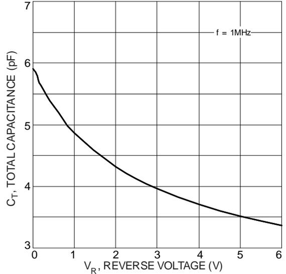
Figure 2 Typical Total Capacitance vs. Reverse Voltage
