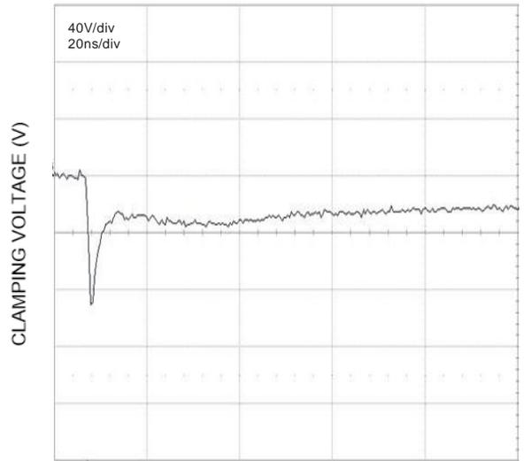
Figure 8 IEC 6100-4-2 Clamping Voltage
