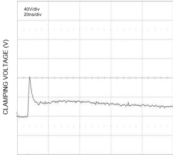
Figure 7 IEC 6100-4-2 Clamping Voltage
