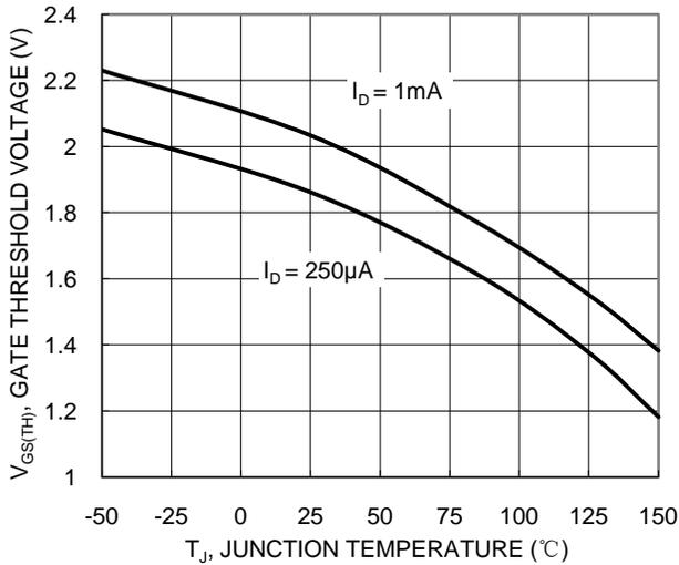
Figure 7. Gate Threshold Variation vs. Junction Temperature
