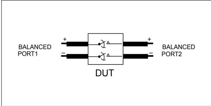
Figure 1. Differential Insertion Loss Setup
