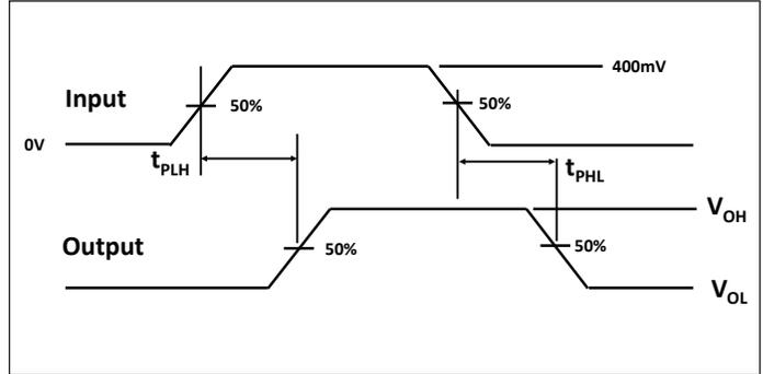
Figure 2. Propagation Delay
