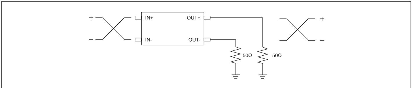
Figure 4. Test Circuit for Propagation Delay
