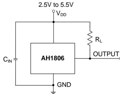
Note: 4.  $C_{IN}$  is for power stabilization and to strengthen the noise immunity, the recommended capacitance is 10nF to 100nF.
