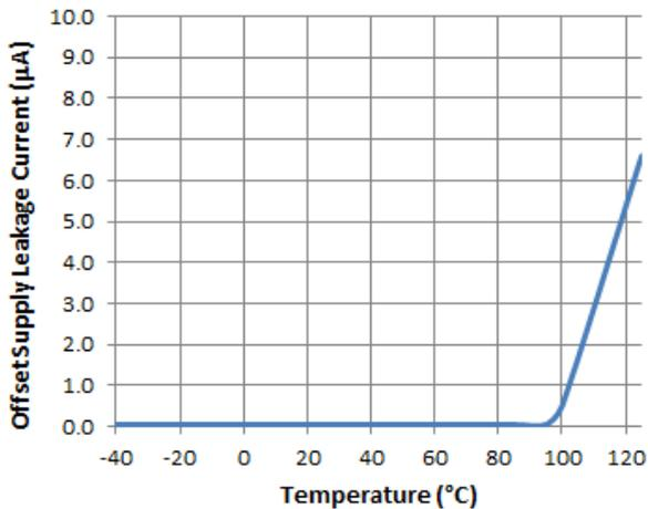
**Figure 26.** Offset Supply Leakage Current vs. Temperature
