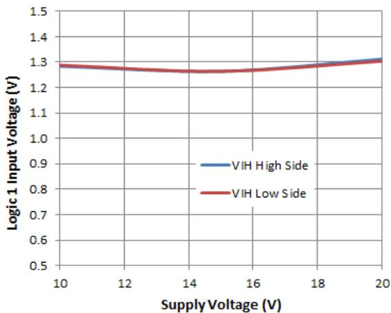
**Figure 20.** Logic 1 Input Voltage vs. Supply Voltage
