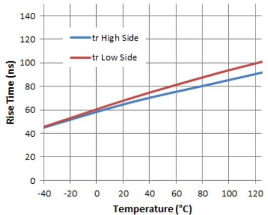
**Figure 9.** Rise Time vs. Temperature
