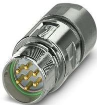
M23, Coupler connector, series: M23 PRO, straight, shielded: yes, for standard and ONECLICK fast locking system, No. of pos.: 7, Direction of rotation: Standard, contact connection type: Pin, Crimp connection, cable diameter range: 9 mm ... 15 mm, coding: N, Item is lead-free in accordance with RoHS II without Exemption 6c (Pb < 0.1 %)
