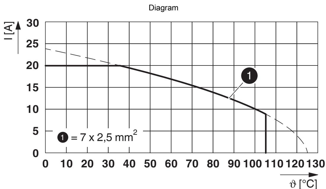
$I$  = current strength,  $\vartheta$  = ambient temperature, 7x 20 A
