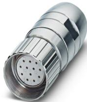
M23, Cable connector, series: UC, straight, shielded: yes, Screw locking mechanism, No. of pos.: 6+3, Direction of rotation: Standard, contact connection type: Socket, Solder cup, cable diameter range: 2 mm ... 14.5 mm, coding: N, Alternative product in accordance with RoHS II without Exemption 6c (Pb < 0.1 %) item no.: 1242191
