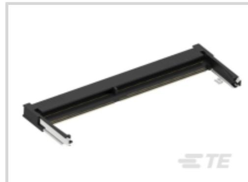
DRAM Type: **Small Outline (SO)**Stack Height: **5.2 mm [.205 in]**Module Orientation: **Right Angle**Number of Positions: **200, 260**Centerline (Pitch): **.5 mm [.02 in]**[All DDR4 SO DIMM Sockets \(39\)](#)**Features****Electrical Characteristics**
