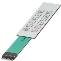
Membrane keypad, self-adhesive, silver conduction technology, 12 keys, embossed, 3 colors, connecting cable: 88.5 mm, with crimp female connector, pitch: 2.54 mm, operating temperature: -20°C ... 70°C
