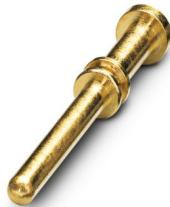
Crimp contact, Pin, turned, contact diameter: 2 mm, crimp range: 0.75 mm<sup>2</sup> ... 1.5 mm<sup>2</sup>,
