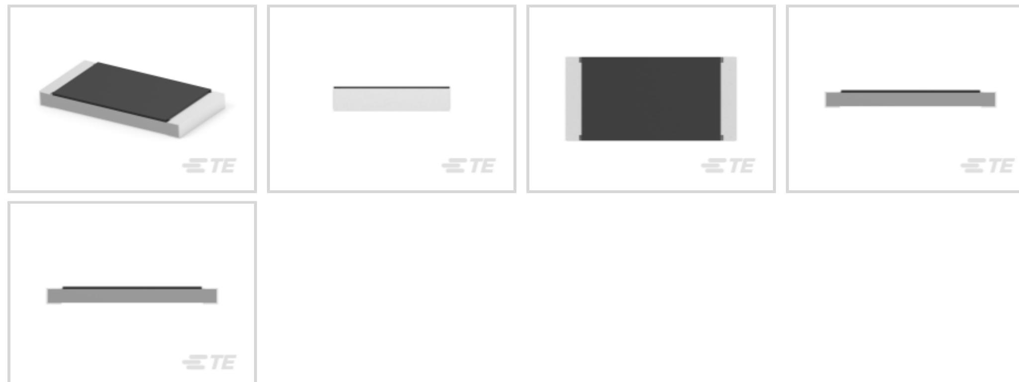
Resistor Type: **Current Sensing Resistor**Element Type: **Thick Film**Package Size Code: **2512**Power Rating: **1 W**Resistance Value: **.027  $\Omega$**
