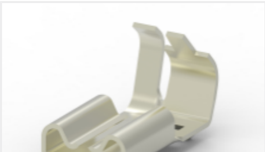
TE Part #2238142-1 250 FASTON,FLAG,REC.,22-16 AWG, NPST
