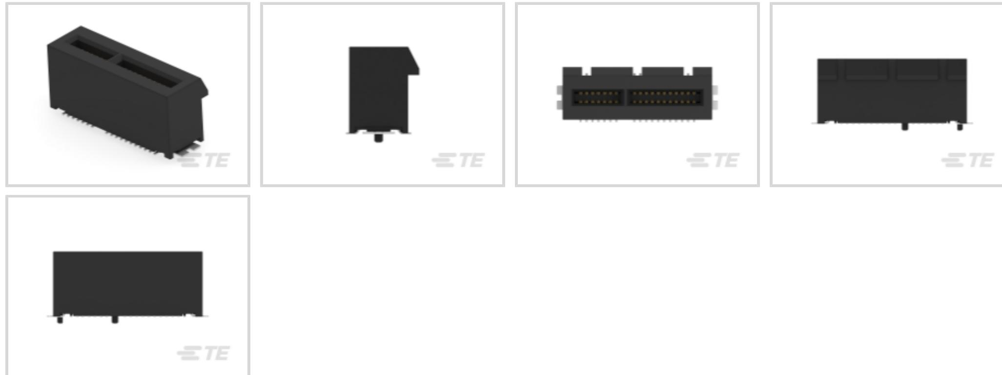
Connector System: **Board-to-Board**Number of Positions: **36**PCI Generation: **5**Centerline (Pitch): **1 mm [.04 in]**Termination Post & Tail Length: **1.1 mm [.043 in]**
