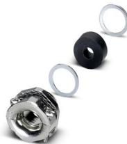
Cable gland, material for screw connection: Brass, nickel-plated, external cable diameter 7 mm .. . 10 mm, shielding: no, connecting thread: Pg9, series: RC
