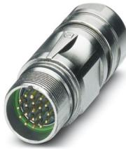
M23, Coupler connector, series: CA, straight, shielded: yes, for standard and SPEEDCON interlock, No. of pos.: 16+2+FE, Direction of rotation: Standard, contact connection type: Pin, Crimp connection, cable diameter range: 4 mm ... 6 mm, coding: N, Alternative product in accordance with RoHS II without Exemption 6c (Pb < 0.1 %) item no.: 1245048
