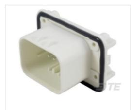
TE Part #776267-2 14POS,PIN DIA 1.3,HDR ASSY,90DEG, COD 2
