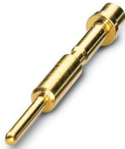
Crimp contact, Pin, turned, contact diameter: 1 mm, crimp range: 0.25 mm<sup>2</sup> ... 1 mm<sup>2</sup>, Alternative product in accordance with RoHS II without Exemption 6c (Pb < 0.1 %) item no.: 1243215
