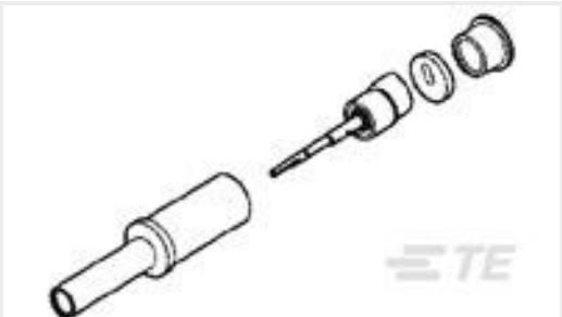
TE Part #1757624-1 SZ 8 COAX PIN, RG142, HEX CRIMP
