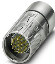
M23, Cable connector, series: M23 PRO, straight, shielded: yes, ONECLICK fast locking system, No. of pos.: 16+2+PE, Direction of rotation: Standard, contact connection type: Pin, Crimp connection, cable diameter range: 4 mm ... 8.5 mm, coding: N, Item is lead-free in accordance with RoHS II without Exemption 6c (Pb < 0.1 %)
