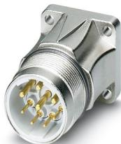
Device connector front mounting, straight, SPEEDCON, M23, number of positions: 5+PE, contact connection type: Pin, Axial O-ring, 4x Ø 3.2, shielded: yes, flange dimensions: 26 mm x 26 mm, number of positions: 6, connection method: Crimp connection, series: SF
