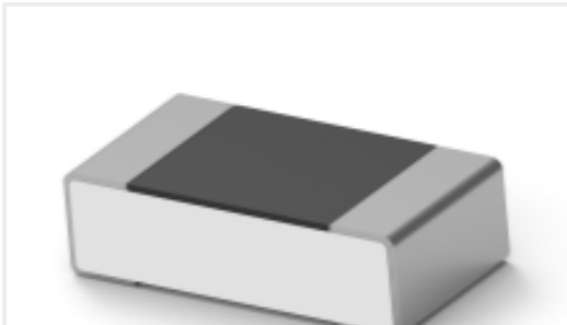
TE Part #2176371-3 RQ 0603 4K87 0.1% 10PPM 5K RL
