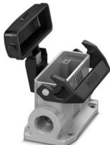
Surface mounting housing D25, with single locking latch, material: Die-cast aluminum, salt water resistant, protective cover material: PC, cable outlets: 2, lateral, 2x M20, height: 57 mm, cable gland: none, protective cover: yes, Standard
