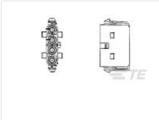
TE Part #794118-1 04P .156 MNL CAP PANEL MOUNT
