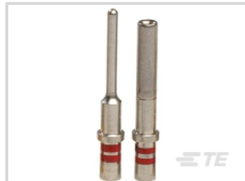
Contact Type: **Socket**Contact Mating Area Plating Material: **Gold**Wire Contact Termination Area Plating Material: **Gold**Contact Size: **Size 20**Wire Size: **24 – 20 AWG**
