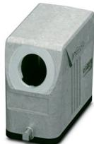
Sleeve housing D15, for single locking latch, material: Die-cast aluminum, salt water resistant, cable outlets: 1, lateral, 1x Pg16, height: 56 mm, cable gland: none, Standard
