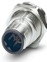
Device connector rear mounting, 4-position, Pin, straight, M12-SPEEDCON, coding: B, Rear mounting, Pg9, Solder pins, Alternative product in accordance with RoHS II without Exemption 6c (Pb < 0.1 %) item no.: 1240087
