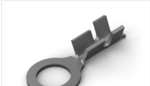
TE Part #170022-2 RING TERMINAL 26-22 AWG 0.140 X .260 BR
