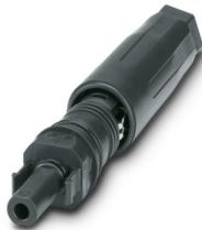
Connector, Range of articles: SUNCLIX, housing material: PPE, color: black, number of positions: 1, min. conductor cross section: 2.5 mm<sup>2</sup>, max. conductor cross section: 6 mm<sup>2</sup>, rated voltage: 1500 V DC, rated current: 35 A, Connection method: Spring-cage, Contact connection type: Socket, min. cable diameter: 5 mm, max. cable diameter: 8 mm
