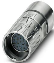
M23, Cable connector, series: M23 PRO, straight, shielded: yes, ONECLICK fast locking system, No. of pos.: 17, Direction of rotation: Standard, contact connection type: Socket, Crimp connection, cable diameter range: 4 mm ... 8.5 mm, coding: N, Item is lead-free in accordance with RoHS II without Exemption 6c (Pb < 0.1 %)
