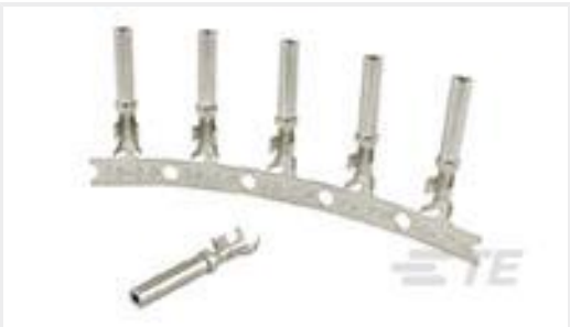
TE Part #1062-16-0722 SOC, SF, SIZE 16, 14-18, NI/SN
