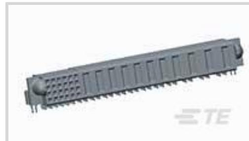
PCB Connector Assembly Type: **PCB Mount Receptacle**PCB Mount Orientation: **Right Angle**Connector System: **Board-to-Board**Number of Positions: **35**Number of Rows: **4****Features****Electrical Characteristics**
