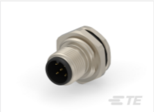
TE Part #T4171010005-001 M12,REAR MOUNTING,MALE,A,5P,0.2 M WIRE
