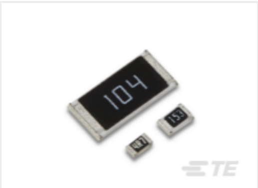
TE Part #4-2176339-5 CRGCQ 0603 47K 1%
