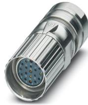
M23, Cable connector, series: CA, straight, shielded: yes, Screw locking mechanism, No. of pos.: 16+2+FE, Direction of rotation: Standard, contact connection type: Socket, Crimp connection, cable diameter range: 6 mm ... 10 mm, coding: N, Alternative product in accordance with RoHS II without Exemption 6c (Pb < 0.1 %) item no.: 1245004
