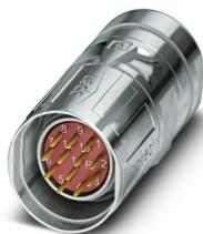
M23, Cable connector, series: CA, straight, shielded: yes, SPEEDCON, No. of pos.: 12, Direction of rotation: Standard, contact connection type: Pin, Crimp connection, cable diameter range: 3 mm ... 14.5 mm, coding: N, Alternative product in accordance with RoHS II without Exemption 6c (Pb < 0.1 %) item no.: 1243589
