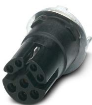
Contact carrier, Ethernet CAT5 (IEC 11801:2002), 8-position, Socket, straight, M12, coding: Y, PCB mounting, THR solder connection, Alternative product in accordance with RoHS II without Exemption 6c (Pb < 0.1 %) item no.: 1239020
